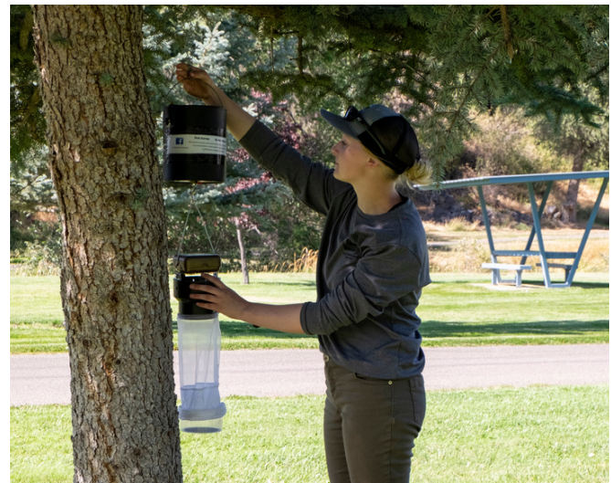
Image 4: Technician setting an EVS trap.
