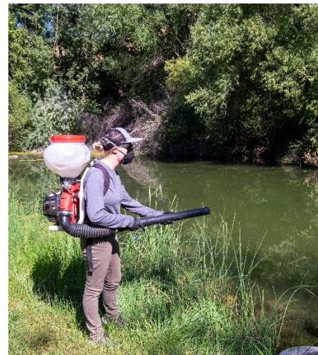
Photo 6: Applying granular larvicide to pond using a Maruyama backpack blower.
